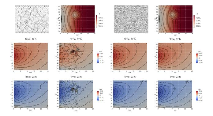
Figure 6: Small amplitude tidal wave. Coarse  $h_K = 100 \, km$  (left block) and fine  $h_K = 50 \, km$  (right block) simulation. Top: mesh and bathymetry. Middle and bottom: snapshot of the free surface at t = 18h and 23h. Left: well balanced scheme. Right: non well balanced scheme. Contour levels are from  $-0.02 \, m$  to  $0.02 \, m$  in intervals of  $0.002 \, m$ .
