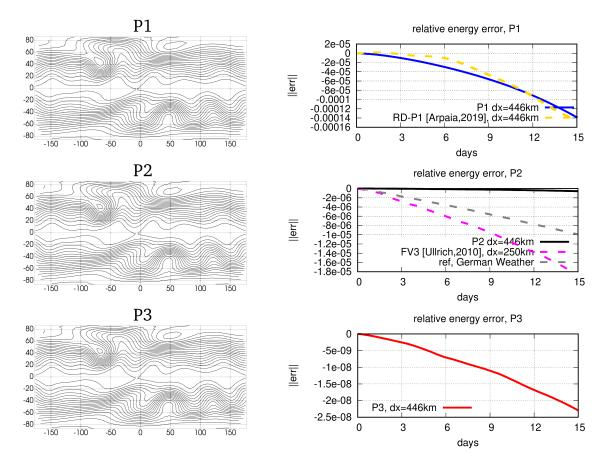
Figure 3: Zonal flow over an isolated mountain. Left: Snapshot at day 15 (depth contour levels from 5050 m to 5950 m-intervals of 50 m). Right: relative energy error (results from 5 32 and from the DWD reported for comparison where relevant)
