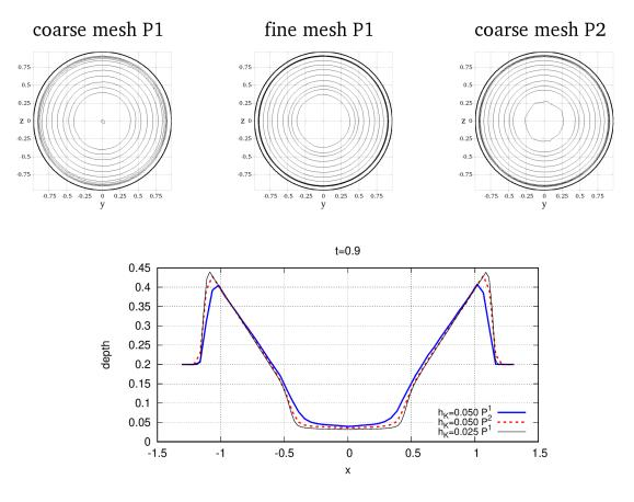
Figure 8: Circular Hump. Contour levels at t = 0.9 from 0.04 m to 0.5 m in intervals of 0.045 m. Bottom: cut along the equator
