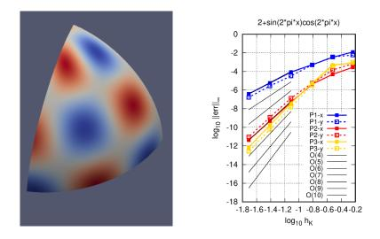
Figure 15: Numerical validation of the well balanced correction estimate for a smooth pressure field. Left: Domain and pressure field. Right: mesh convergence for  $|\epsilon_P^K|_{\infty}$ . The dashed and continuous lines represent the x and y components of the correction.
