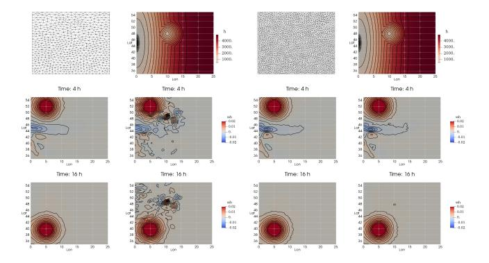
Figure 7: Small amplitude surge wave. Coarse  $h_K = 100 \, km$  (left block) and fine  $h_K = 50 \, km$  (right block) simulation. Top: mesh and bathymetry. Middle and bottom: snapshot of the free surface at t = 4h and 16h. Left: well balanced scheme. Right: non well balanced scheme. Contour levels are from  $-0.02 \, m$  to  $0.02 \, m$  in intervals of  $0.002 \, m$ .
