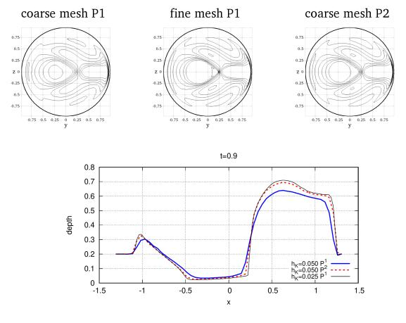
Figure 9: Circular Hump with rotation. Contour levels at t = 1.2 from 0.04 m to 0.5 m in intervals of 0.045 m. Bottom: cut along the equator
