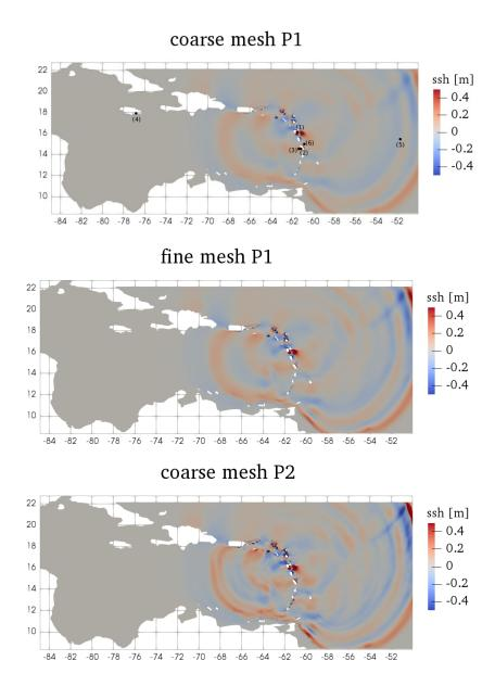
Figure 11: Tsunami in the Carribean Sea. Color map of sea surface height  $\eta$  after 5400 s. Numbers (1) to (6) in the top picture show the position of the six stations considered in Figure 12 which corresponds to: (1) Pointe-a-Pitre, (2) Fort-de-France, (3) Martinique W, (4) Kingston, (5) Atlantic Ocean, (6) Martinique NE.
