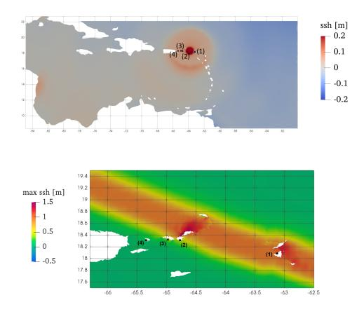
Figure 13: Hurricane Irma. Top: color map of the simulated surge the 06/09/2017 14:00:00. Bottom: close up view of the maximum water surface elevation in the region of Puerto Rico. Numbers (1) to (4) show the position of the four stations considered in Figure 14 which respectively correspons to: (1) Saint Martin, (2) Lameshur Bay, (3) Charlotte Amalie, (4) Culebra locations.
