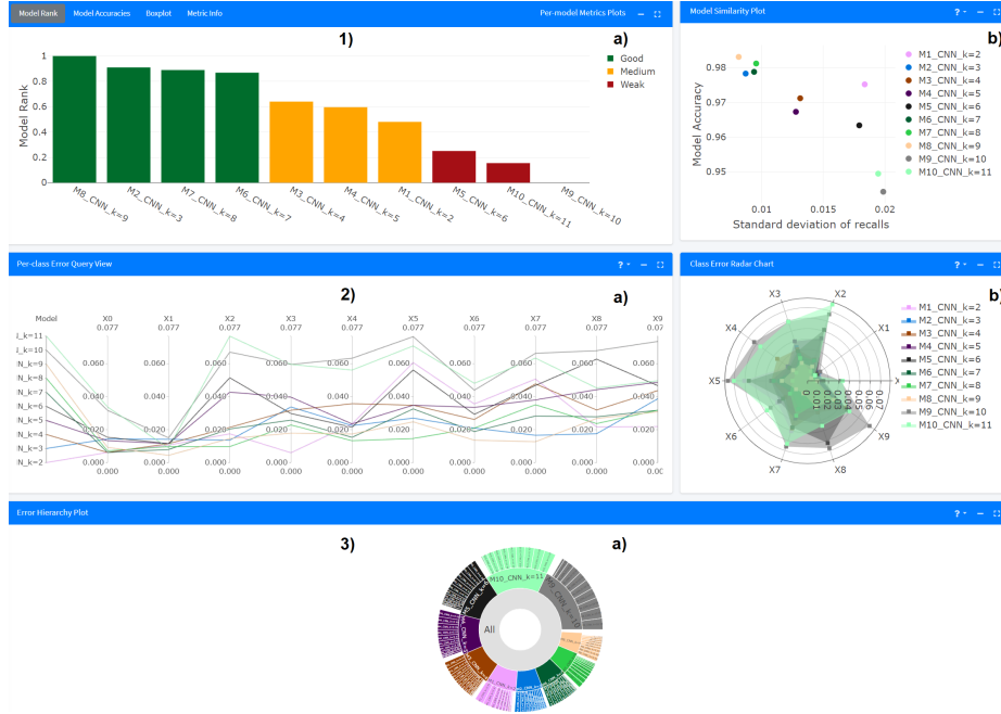
Fig. 1. Model overview pane contrasting the results of ten multi-class classifiers on the MNIST data set. The models are ranked according to their accuracy and classification imbalance in 1) a). The non-monotonic effect of the varied kernel size in the used convolutional neural networks can be seen in 2) a).
