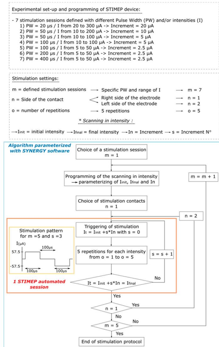
**Figure 3.** Algorithm illustrating parameterization of SYNERGY software to implement Protocol 1. Protocol 1 was designed to perform scanning in intensities with different pulse widths using a TIME implanted in a single fascicle (TIME#1). This experiment was implemented to ensure STIMEP ability to automatically deliver finely tuned stimulations but also to assess the relative impact of both intensity and pulse width in intrafascicular stimulation selectivity.
