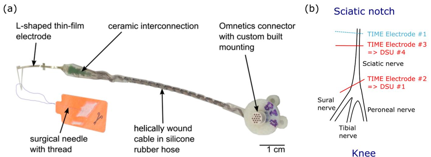
**Figure 2.** Transverse Intrafascicular Multichannel Electrode (TIME) and implantation procedure. (a) Photograph of the TIME-4H implant. Each TIME consists of 14 independent stimulation contacts and 2 ground sites. (b) Implantation of TIME devices into the sciatic nerve proximal to its trifurcation at the knee especially for protocol 2.
