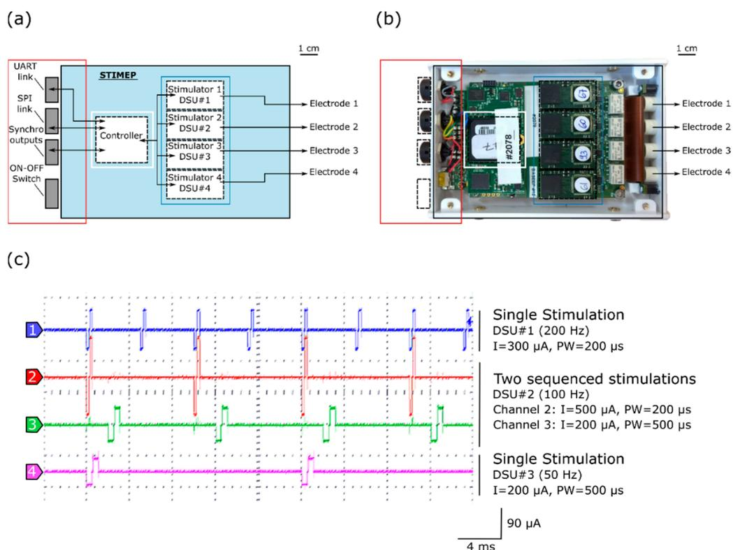
**Figure 1.** STIMEP architecture and bench testing. (a) Diagram of STIMEP hardware and (b) picture of the corresponding device at the same scale. (c) Coordinated DSU stimulations with different frequencies, intensities and pulse widths (oscilloscope screenshot).
