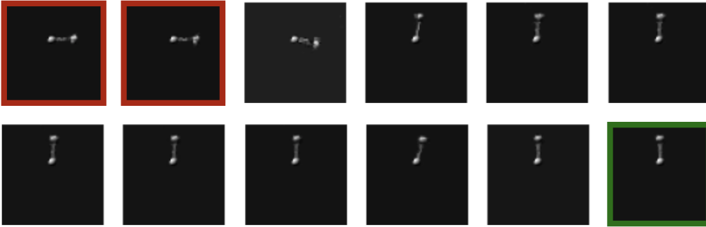
Figure 6: Illustration of pendulum control. Starting from two consecutive configurations (in red), control inputs are applied to the pendulum to force it to be in an inverted position in a horizon of 0.5 s. Final position is the target configuration (in green).
