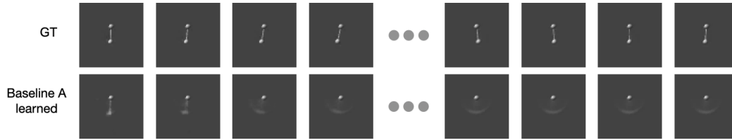
Figure 9: Prediction for the pendulum with low oscillations amplitude (between \frac{\pi}{2} and \frac{3\pi}{2} radians) with lengths varying from 0.3 to 0.8 m. The first row shows ground truth (GT) images. The second row shows predicted frames with the baseline model where the matrix A is a learned parameter.
