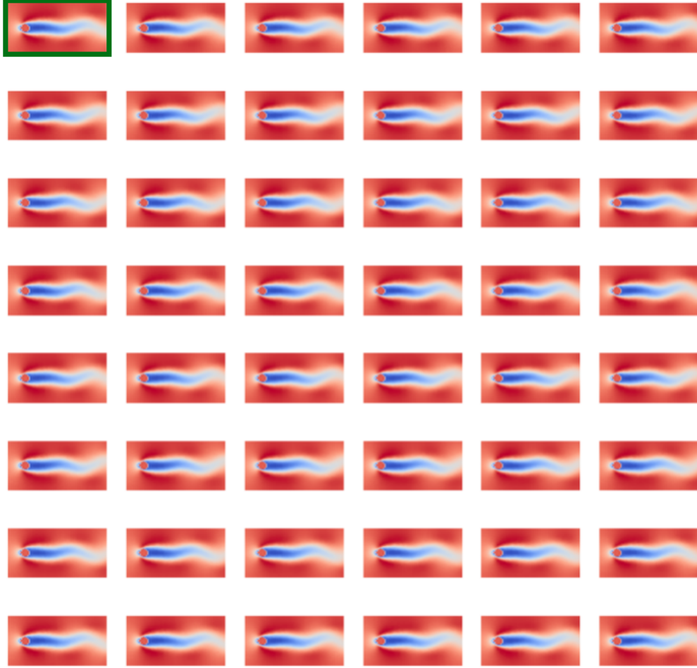
Figure 15: Prediction of the x-momentum. The top-left frame is the last frame of the 16 frame-long sequence that was used to build the dynamics matrix A . All the following frames are predicted.
