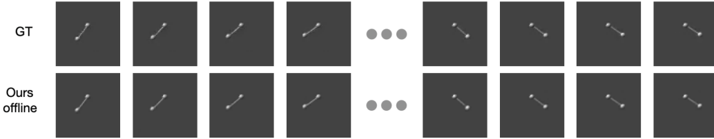
Figure 7: Prediction for the pendulum with low oscillations amplitude (between \frac{\pi}{2} and \frac{3\pi}{2} radians) on a dataset of pendulums of length varying between 0.3 m and 0.8 m. The first row shows ground truth (GT) images. The second row shows predicted frames with our model without updates. In the case of this simple system, our model without updates is enough.
