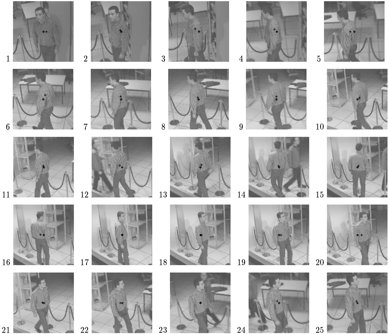
Figure 9: Tracking of a pedestrian. An image upon ten of the acquired sequence (approximately 2 frames per second). Cross (+) stands for the estimated c.o.g. and diamond ( \diamond ) for the image center
