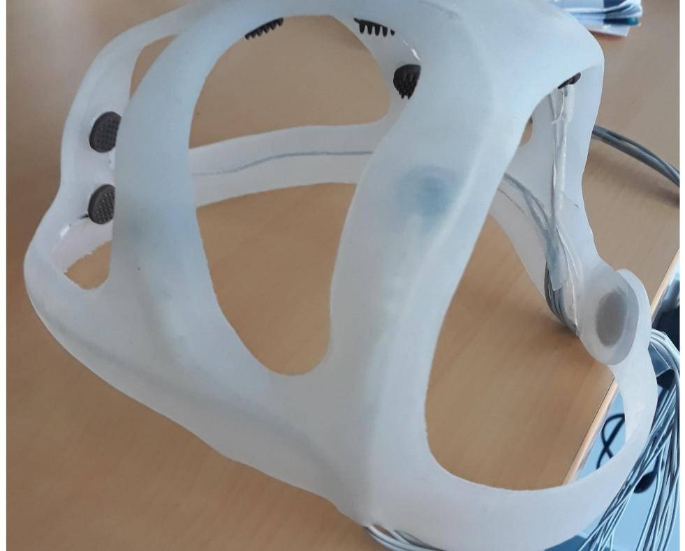
Impedance analysis (1h) for the working mode explicited by Fiedler [4], revealed that our prototype stand with a mean impedance of 50 k $\Omega$  and a variability of 71.6 k $\Omega$  (see Fig.3), with the worst contact being 534 k $\Omega$ , still in the 1M $\Omega$  range
