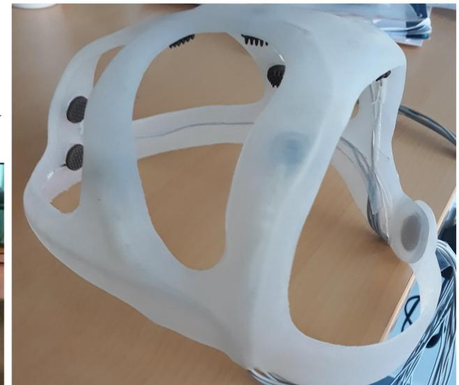
**Impedance analysis** (1h) for the working mode explicated by Fiedler [4], revealed that our prototype stand with a **mean impedance of 50 kΩ** and a variability of 71.6 kΩ (see Fig.3), with the worst contact being 534 kΩ, still in the 1MΩ range defined by literature.
