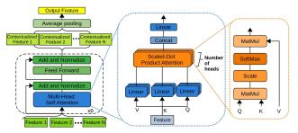
Figure 4. (Left) Our view fusion module. (Middle) Multi-Head Attention module. (Right) Scaled Dot-Product Attention.
