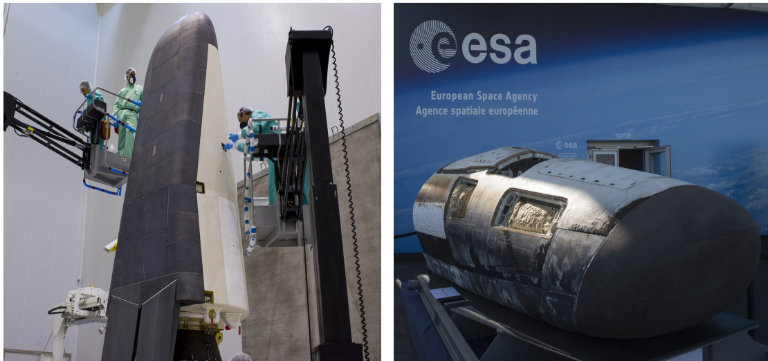
Figure 2: IXV before and after atmospheric re-entry : mechanical and thermal stresses can be noticed on the side of the spacecraft on the TPS. Note that the nose has been restored for exposure. Credits to ESA 1,2
