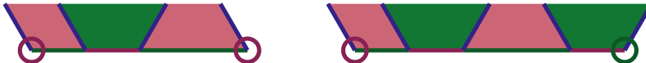
Figure 4: Examples of even and odd blue boundaries. On the left a blue boundary joining two red corners. It has an even length and should therefore be considered as a stabilizer. On the right a blue boundary joining a red corner and a green one. It has odd length and will not be measured by the schedule of measurements.
