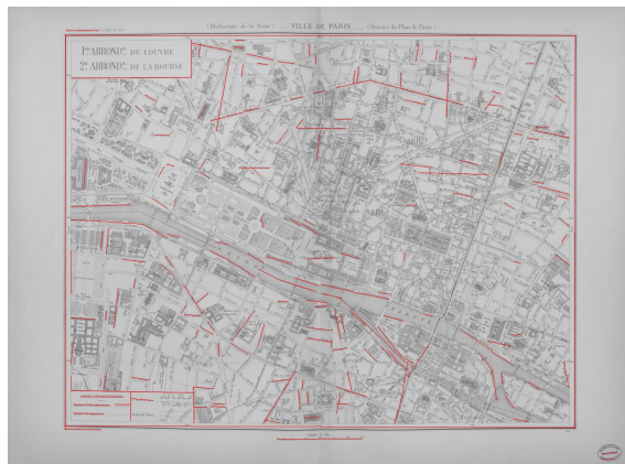
Fig. 3. Line segment extraction at low resolution: visual clues for map outer frame detection (181 detected segments)
