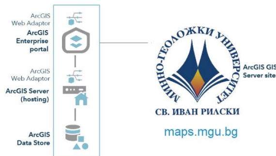
Fig. 10. Architecture of the geoinformation portal of University of Mining and Geology "St. Ivan Rilski" (Sofia, Bulgaria), [Source (with modifications): https://enterprise.arcgis.com/en/get-started/latest/windows/additional-server-deployment.htm ]
