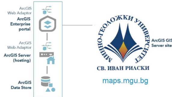
Fig. 10. Architecture of the geoinformation portal of University of Mining and Geology "St. Ivan Rilski" (Sofia, Bulgaria), [Source (with modifications): https://enterprise.arcgis.com/en/get-started/latest/windows/additional-server-deployment.htm ]
