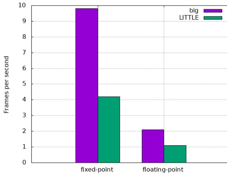
Figure 3: Impact of fixed-point representation on FPU-less processors
