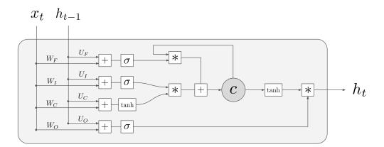
Figure 3.4: Illustration of an LSTM unit, a typical example of recurrent layer. The layer outputs a vector  $h_t$  (for the  $t^{th}$  term of the sequence) and takes its last output  $h_{t-1}$  as an additional input.
