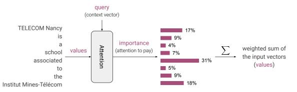
Figure 3.5: Simplified diagram of the operations performed by an attention layer. In practice, words are embedded into latent vectors. This is why we can carry out a weighted sum of *words*.
