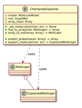
Figure 5.3: Simplified class diagram of the solution.
