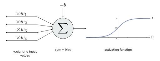
Figure 3.2: Pipeline of an artificial neuron, the perceptron
