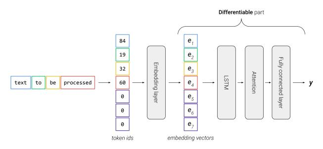
Figure 4.8: Neural network architecture used for text classification
