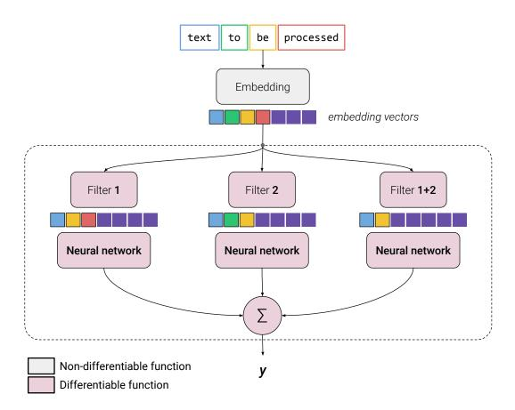
Figure 4.11: Illustration of the proposed solution, EnsembleOut with filters directly applied on embedding vectors<sup>19</sup>
