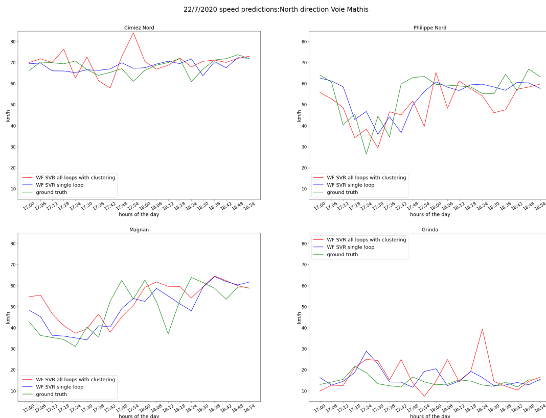
Figure 28: Speed predictions on 22/7/2020, "Walk Forward SVR single loop" and "Walk Forward SVR all loops with clustering".
