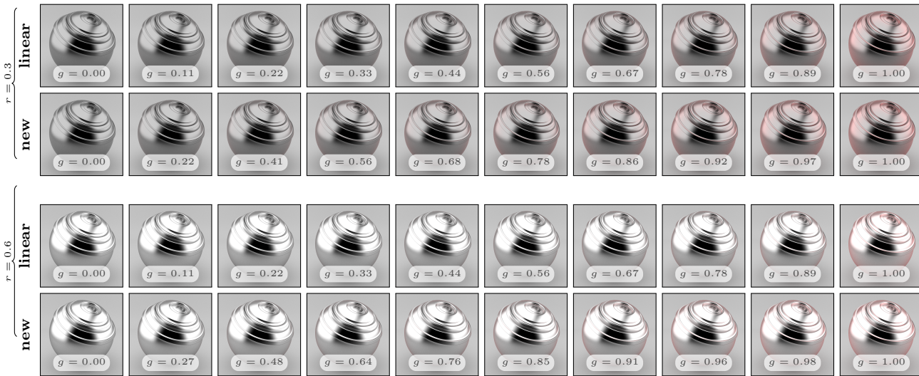
Figure 6: Results for complex refractive index remapping. We display results of a linear range of edge-tint values for a low ( r = 0.3 ) and high ( r = 0.6 ) reflectivity setting. Compared to renderings using Gulbransen’s parameterization ( r, g ) (top rows), our new mapping ( r, g' ) (bottom row) better distributes the redish edge tint effect. The associated g value is displayed for each configuration.
