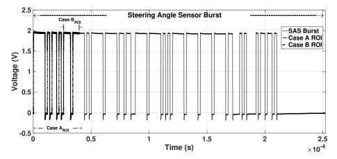
Figure 3. Data frame or burst from a Toyota SAS.
