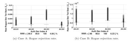
Figure 12. Rejection rates of a device (A4) using the credentials of other devices.
