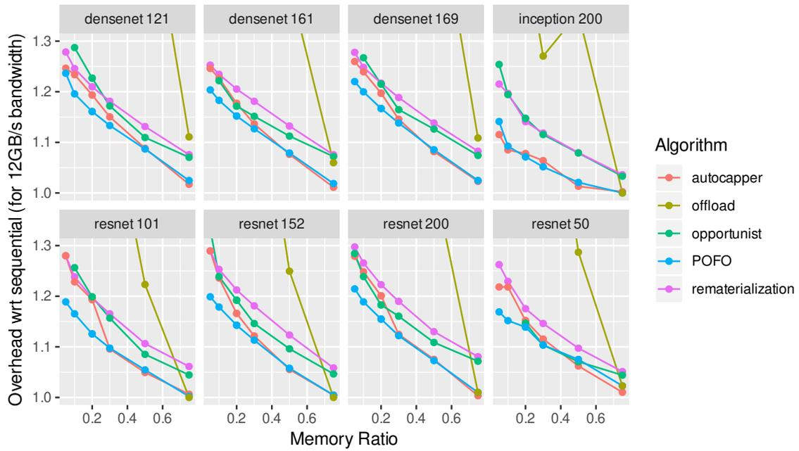
Figure 2: Simulation results for fixed bandwidth  $\beta = 12\text{GB/s}$  and varying memory ratio  $\alpha$ .
