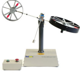
Fig. 1. TRMS 33-220 twin rotor MIMO system
