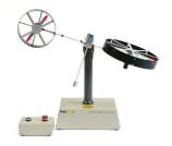
Fig. 1. TRMS 33-220 twin rotor MIMO system
