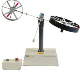
Fig. 1. TRMS 33-220 twin rotor MIMO system
