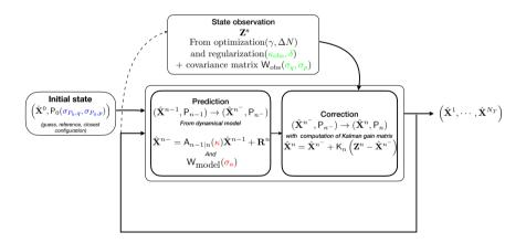
Fig. 5 The parameters of the Kalman filter and the state observation.
