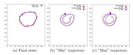
**Fig. 14** Simulation for  $\sigma=2.0$ ,  $\sigma_v=0.003$ ,  $\sigma_q=1.5$ . Red : real vesicle. Blue : estimation by the method.  $\kappa=10$ ,  $\kappa_{\rm obs}\delta=0.1$ .
