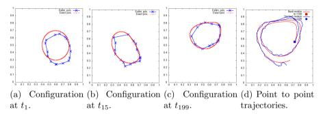
Fig. 21 Vesicle configuration (blue) at  $t_n$ , n=1,69,199 against the solution (red). Right hand side: trajectory of a point in the estimation (blue) compared to the one of the presumed tracked point in the real vesicle (red) at final iteration. Parameters:  $\kappa=10,\kappa_{\rm obs}\delta=0.0,\sigma=6.0,\,\sigma_v=0.075$ .
