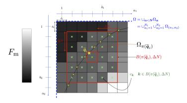
Fig. 4 Two-dimensional illustration of optimization step parameters in the position observation operator ( $\Delta N=2$ ). The landmark (mesh point) i is in  $\tilde{q}_i(t)$  in the prior mesh (yellow). It is inside the voxel  $\Omega_{\pi(\tilde{q}_i)}$  (in red) which defines the local window search  $B(\pi(\tilde{q}_i(t)), \Delta N)$  for the optimum. The functional  $J_t(\tilde{q}_i; \cdot)$  will be evaluated in the voxel centers  $c_k$  for all  $k \in B(\pi(\tilde{q}_i(t)), \Delta N)$ .
