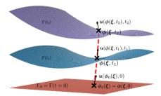
**Fig. 1** Illustration of the transport of  $\Gamma(t)$  through the velocity field u.
