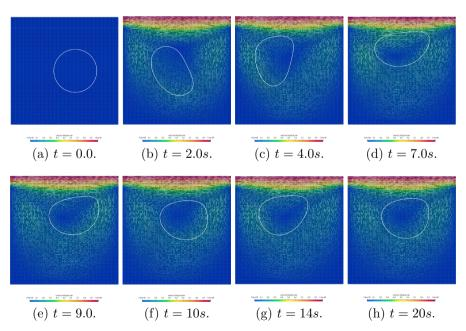
Fig. 7 Data generation - Motion of the immersed vesicle, from FSI simulations.
