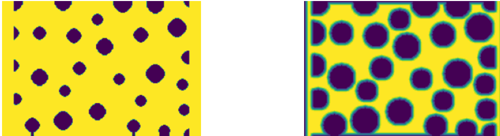
(a) Dilation using a flat square structuring element (b) Erosion using a Gaussian structuring element
