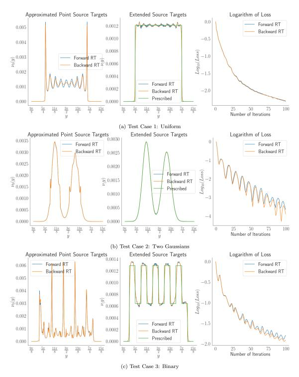
Figure 9: Comparison of forward/backward ray tracing
