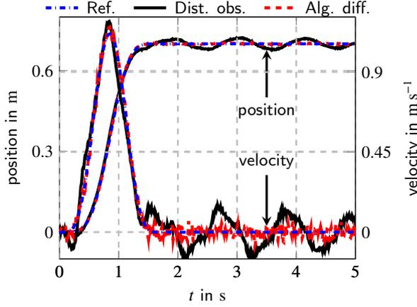
Figure 4: Time evolution of position and velocity.
