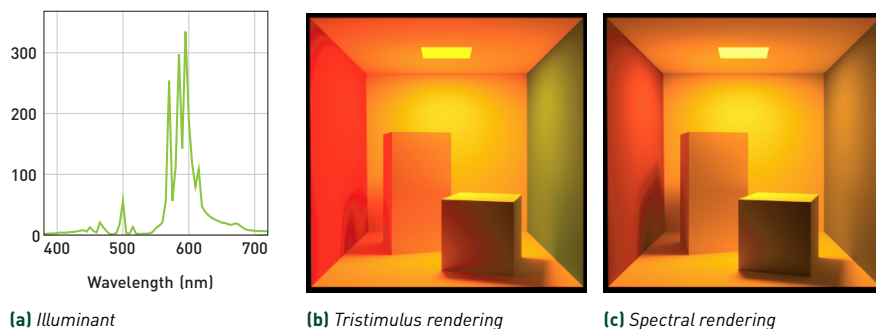
Figure 42-3. Discrepancies induced by a tristimulus renderer are even more prevalent in a global illumination context. This leads to important color and intensity differences, especially with narrow spectra like the one used to light this Cornell box scene (HP1, high-pressure vapor lamp).
