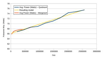
Fig. 11. Power depending on gas consumption
