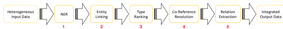
Fig. 1. The XI Pipeline goes through a series of five steps to integrate semi-structured or unstructured content leveraging a Knowledge Graph
