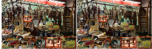
Figure 2: Proof of concept for extreme \times 16 upsampling. The right image is obtained by processing a burst of 20 LR images presented on the left obtained with synthetic random affine movements and bilinear downsampling.
