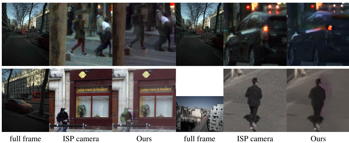
Figure A8: Misalignments artefacts due to moving objects in the scene. Our current implementation does not handle fast moving objects and then generates visual artefacts. Dealing with fast dynamic scenes will be the focus of future work.
