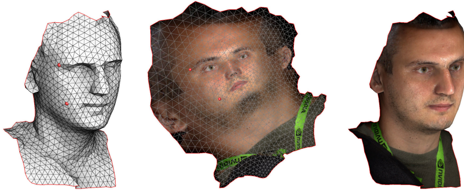
Figure 6.8: Least squares conformal mapping. Left: input mesh; middle: unfolded mesh textured by an artist; right: final textured surface. Two pinned vertices are shown in red.
