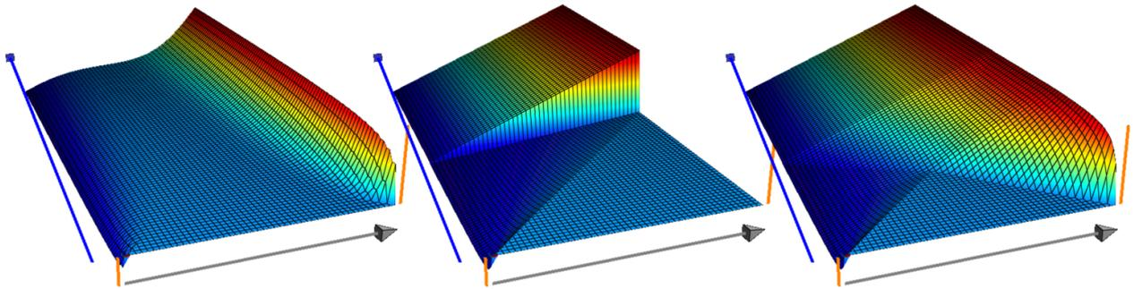
Figure 7.10: Evolution of the solution with  $n = 20$ : the gray axis represents the function sampled by  $x$ , and the blue axis is the iteration axis, the orange segments are the boundary constraints. Three solvers are (from left to right) the gradient descent, the conjugation and the conjugated gradient.
