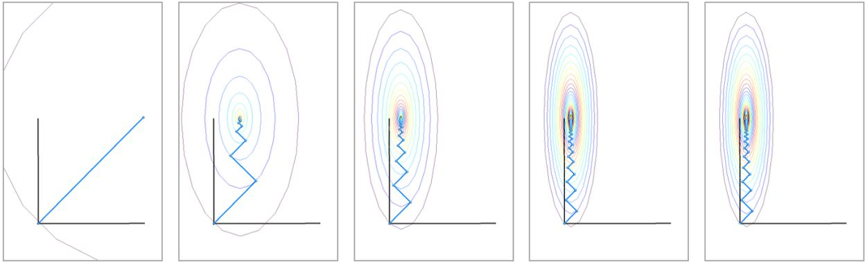
Figure 7.2: Optimal step gradient descent with a diagonal matrix  $A$ , where  $a_{00}$  takes values from 1 (left) to 5 (right),  $a_{11} = 1$  and  $a_{10} = a_{01} = 0$ . The blue segments connect the  $x^{(k)}$  to the  $x^{(k+1)}$ , and the ellipses show the iso-values of  $f(x) = x^T Ax - 2b^T x$ .
