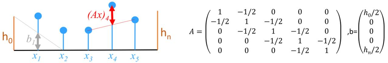
Figure 7.9: 1D Laplacian problem. We have a function defined in  $n = 5$  points; the goal is to minimize the second derivative estimated by finite differences i.e.,  $\sum_i (x_i - (x_{i-1} + x_{i+1})/2)$ . At the boundary we fix values  $h_0$  and  $h_n$ , which gives the problem  $Ax - b = 0$  with  $A$  and  $b$  shown in the figure.
