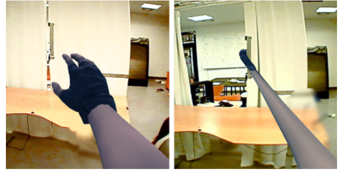
Fig. 3. Example of partial avatarization with a head-mounted VST display (Feuchtner and Müller [57]). Left: A virtual arm of normal length is embodied in first-person AR. Right: The user extends his virtual arm towards a normally unreachable (real) electric curtain and manipulates it.
