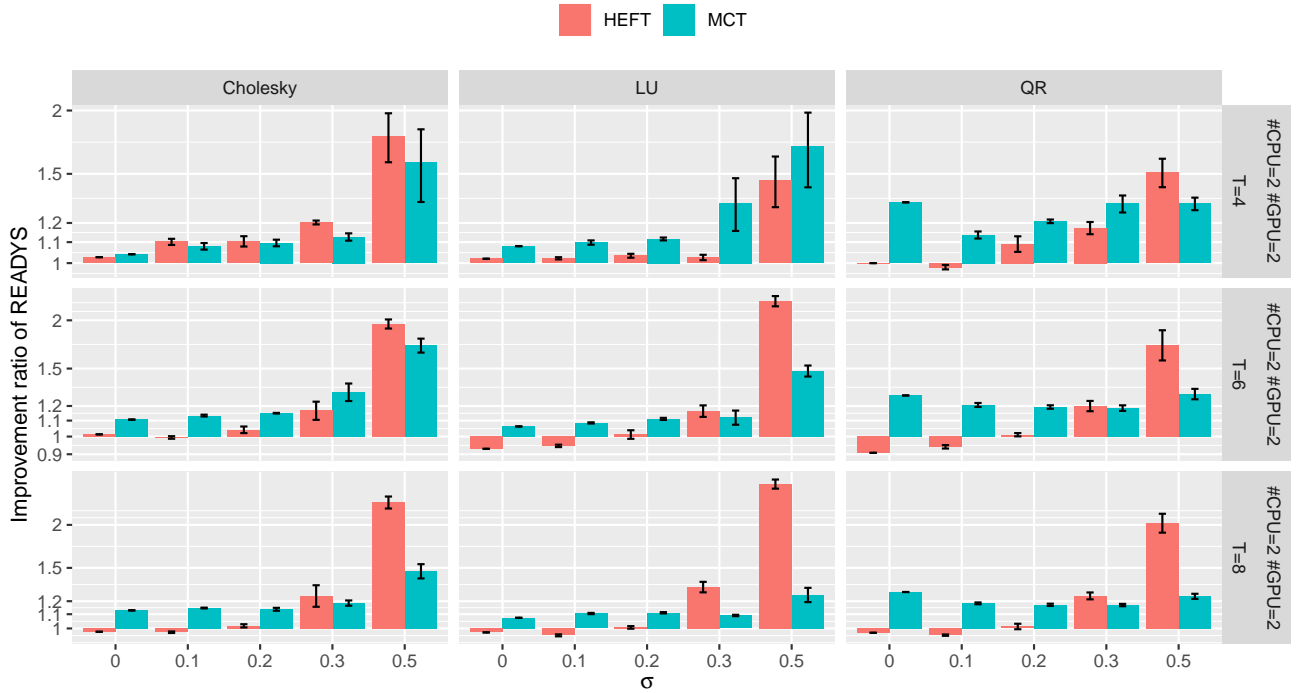
Figure 3. Makespan improvement over HEFT and MCT according to T \in \{2, 4, 8\} (rows), the noise level \sigma , and for each of the 3 tasks we consider (3 columns), when the computing platform is made of 2 CPUs and 2 GPUs. The larger the bars above 1, the better READYS performs w.r.t. to competitors.
