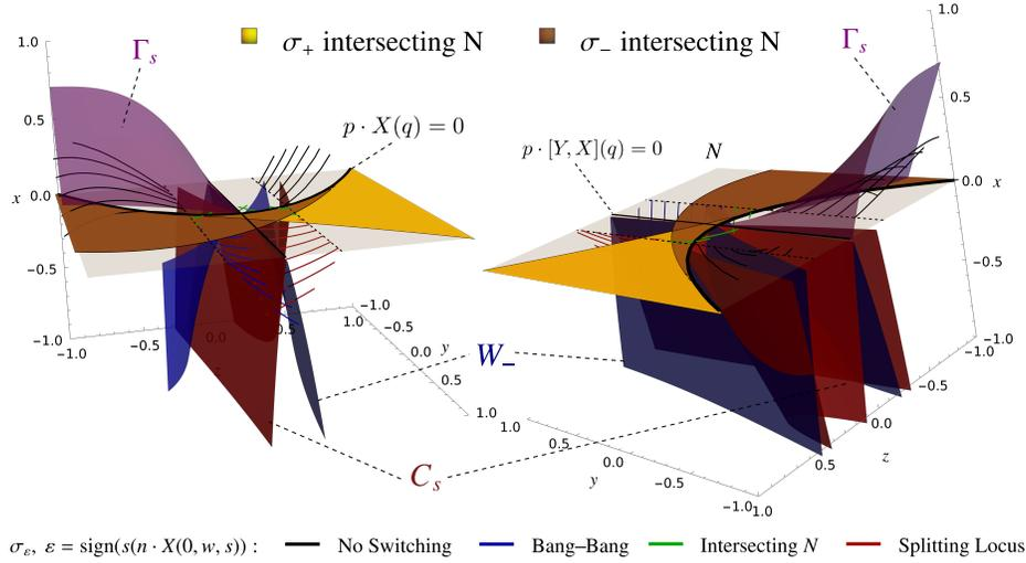
FIGURE 8. Strata of the surface  $S$  separating the regions of  $U$  where the control is  $\pm 1$  for the model (18) with  $b = b_1 = 1$ ,  $c = 0$ . We also represent the regions where  $\sigma_\pm$  intersect  $N$  for  $t < 0$  and several trajectories which generate a switching locus and a splitting locus.
