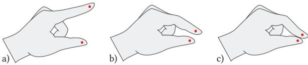
**Figure 2: The interpretation of users’ hand movements in the air depends on the distance  $\Delta_{TI}$  between the thumb’s tip and the index finger’s tip. a) Out of Range ( $\Delta_{TI} > 4\text{cm}$ ): hand movements have no effect; b) Tracking ( $2\text{cm} < \Delta_{TI} < 4\text{cm}$ ): hand movements control which widget is in focus; c) Dragging ( $\Delta_{TI} < 2\text{cm}$ ): hand movements actually control the widget in focus.**
