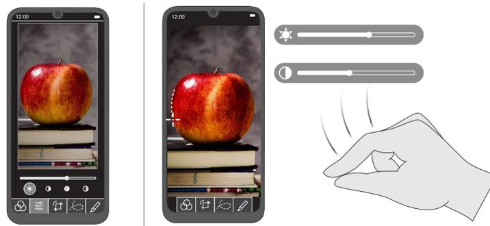
**Figure 7: Redesign of the image editing application from Figure 1 following the guidelines derived from our empirical results. Buttons remain on the smartphone. Sliders for parameter adjustments performed frequently get offloaded. 2D selection can be performed directly on the phone, or indirectly in the air (dual-precision mode) if occlusion is an issue.**
