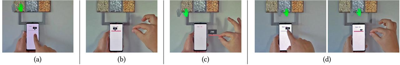
**Figure 4: The four techniques tested in Experiment E<sub>2</sub>: a) *Screen - Screen* ( $CD \mathcal{L}$ ), b) *Screen - Air* ( $CD \mathcal{L}$ ), c) *Air - Air* ( $CD \mathcal{L}$ ), d) *Screen - Screen+Air* ( $CD \mathcal{F}$ ), performing a coarse selection on the touchscreen (left), then a precise adjustment in the air (right). The two hand icons provide basic feedback about HoloLens left & right hand tracking status and never interfere with widgets displayed in the air.**
