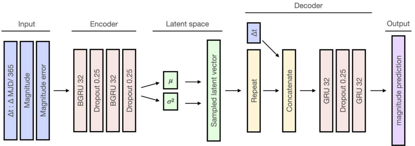
**Figure 4.** Proposed VRAE architecture. The model receives as input  $\Delta t$ , normalized magnitude, and the normalized magnitude error, and outputs a prediction of the normalized magnitude for the original  $\Delta t$  vector.
