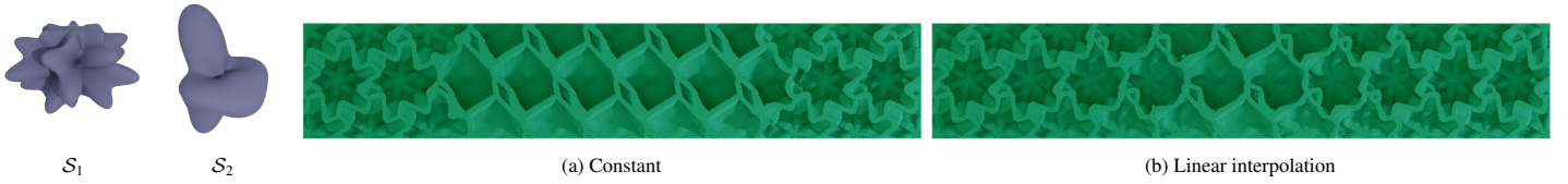
Figure 10: Closed-cell geometry gradation: central part with \mathcal{S}_2 and the rest with \mathcal{S}_1 .
