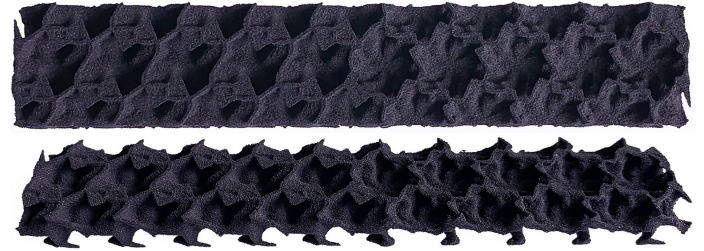
Figure 17: 3D printed, progressive gradation between two closed-cell materials.
