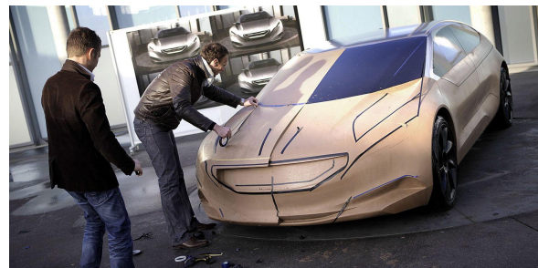
Figure 1: Designers using black tape to visualize the desired feature lines [Courtesy Peugeot Design Lab http://www.peugeotdesignlab.com/fr/le-studio/concept-cars/peugeot-hx1 ].
