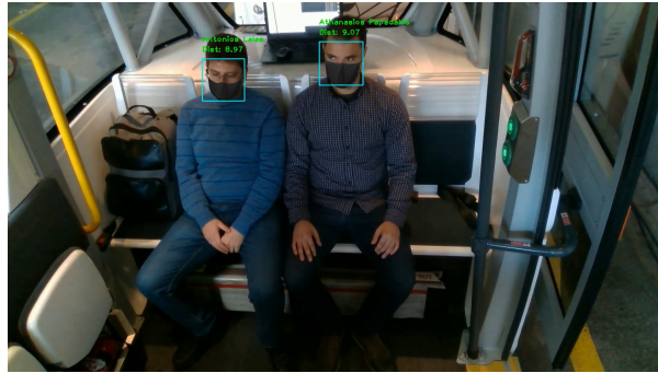
Fig. 4. An experimental real-world demonstration running on the NVIDIA Jetson AGX Xavier. The proposed system is able to correctly identify the two passengers of the autonomous shuttle, among a database of 20 people.
