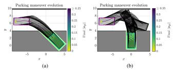
Fig. 9. Constrained non-parallel forward parking maneuvers: (a) diagonal and (b) perpendicular. Initial pose =  $(-8 \text{ m}, 6.5 \text{ m}, 0^{\circ})$
