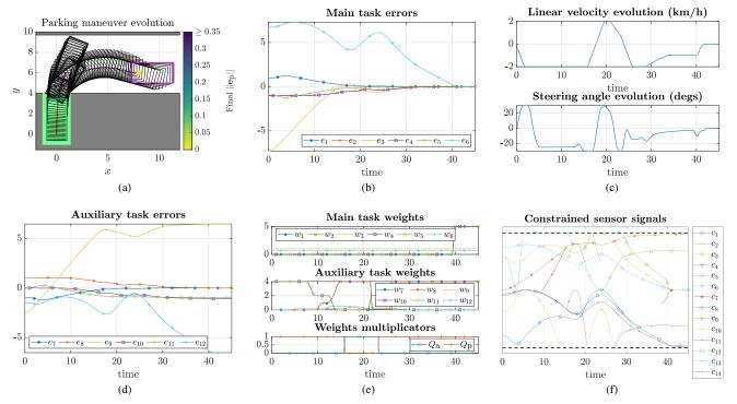
Fig. 6. Constrained  $\perp$  backward parking maneuver signals: (a) performed maneuver, (c) control signals, (e) weighting-related signals, (b) main and (d) auxiliary task errors and (d) constrained sensor signals. Initial pose =  $(8 \text{ m}, 6 \text{ m}, 0^{\circ})$
