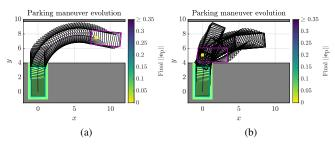
Fig. 7. Constrained  $\perp$  backward parking maneuvers. (a) Initial pose =  $(8 \, \text{m}, 7.5 \, \text{m}, -5^{\circ})$ , (b) Initial pose =  $(0 \, \text{m}, 5.1 \, \text{m}, 0^{\circ})$
