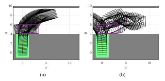
Fig. 13. RRT\* path planning results using  $HC^{00}$ -RS steering function. Initial pose =  $(0m, 5.1m, 0^{\circ})$
