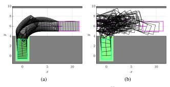
Fig. 11. RRT\* path planning results using  $HC^{00}$  steering function. Initial pose =  $(8m, 6m, 0^{\circ})$
