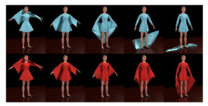
Fig. 13. Corresponding frames of a simulated character displaying cloth on cloth friction. Top Row: M02 (Polyester 95 %, Spandex 5 %) with  $\mu = 0.3$ , Bottom Row M06 (100 % Polyester) with  $\mu = 0.7$
