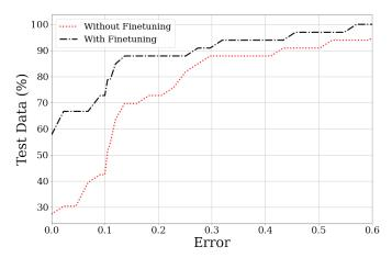
Fig. 11. Prediction errors on Cloth to Cloth friction test dataset
