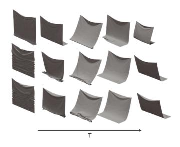
Fig. 1. Three cloth motion sequences simulated with the same material but different friction coefficients at contact ( $\mu$ ). Top:  $\mu = 0.0$ , Centre:  $\mu = 0.5$ , Bottom:  $\mu = 0.6$ . Differences are significant between  $\mu = 0.0$  and  $\mu = 0.5$ , but more subtle between  $\mu = 0.5$  and  $\mu = 0.6$ .
