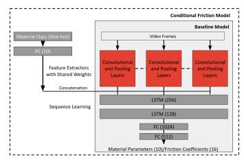
Fig. 5. Proposed architecture to estimate friction conditioned on material parameters. The coloured inlay shows the baseline model, which is augmented with material class information to form the conditional friction model.
