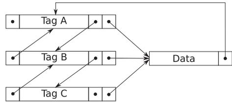
Fig. 2. A generic tag-data doubly linked list. Each tag entry has extra metadata to inform which are the previous entry, next entry, and corresponding data block. Each data entry contains a pointer to the head of its corresponding tag list.
