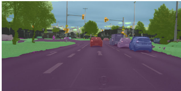
Fig. 1. Output from YOLO-Panoptic on an image from the Cityscapes Dataset.
