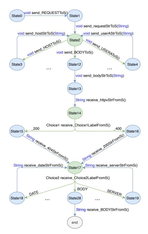
Fig. 1. State machine for CProtocol
