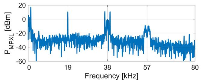
Fig. 4. Example of received high priority warning signal (baseband)
