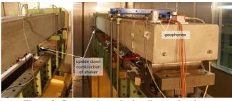
Figure 2. Concrete beam in the climate chamber.
