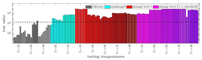
Figure 5. Test values at different testing temperatures in the undamaged state and at two damage levels. Averaged reference null space and covariance matrix are computed from a merged data set recorded at -25°C, 5°C, and 40°C.
