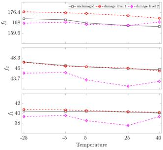
Figure 3. 1<sup>st</sup> to 3<sup>rd</sup> eigenfrequencies at different system states and at different temperatures. The y-axis is scaled to about 5% of each frequency.
