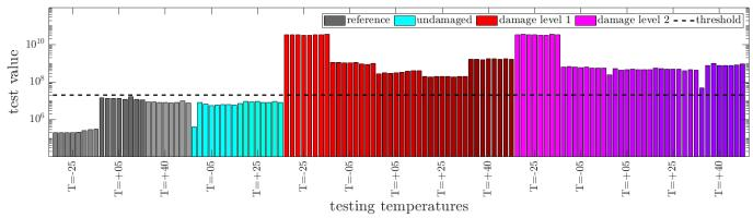
Figure 6. Test values at different testing temperatures in the undamaged state and at two damage levels. **Interpolated** reference null space and covariance matrix are computed from local matrices at -25°C, 5°C, and 40°C.
