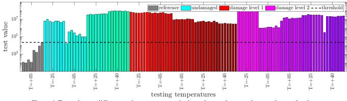
Figure 4. Test values at different testing temperatures in the undamaged state and at two damage levels. **Fixed** reference null space and covariance matrix are computed with data from one data set recorded at 5°C.
