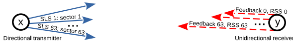
Figure 2: A Sector Level Sweep (SLS) phase in IEEE 802.11ad. The transmitter successively sends one SLS frame per sector . The receiver reports back the per-frame Received Signal Strength (RSS) values.
