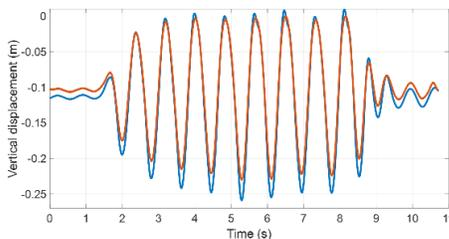
Figure 2 Experimental (blue) and numerical (red) vertical displacements at the diving board free edge
